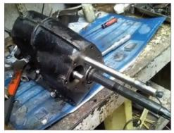
roll pin through the side of it. You will need to make up a dummy layshaft (I use an old layshaft cut down to size) this will need to be slightly shorter than the lay gear and must be inserted into the laygear from the front driving the existing layshaft out of the rear (see pic). The layshaft will then drop into the bottom of the gearbox and the dummy shaft will hold the
