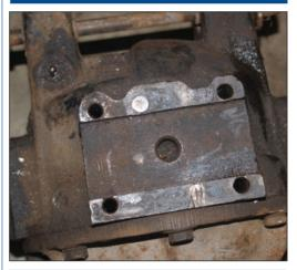
4 Stud Diff casing – Used on Swing Spring Cars only. Note the blanking plugs where the centre 2 studs would be on a 6 stud casing
