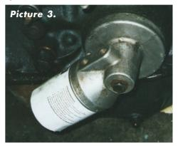
Moving on to a request from a Club member for the type number of oil filter used on the spinon-conversion fitted to the Vitesse 2 Litre engine. The Unipart type number is GFE180, the Champion C104 and Halfords HOF200. This filter was used by a number of motor manufacturers back in the 1980's and should still be ready available.
