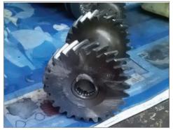
needle bearings in place (pic2). Next we must remove the input shaft, I have
