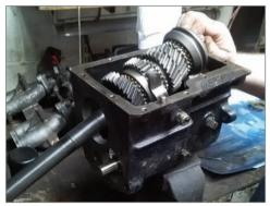
mainshaft has to be tilted to remove it from the box(see pic) and getting to this stage is hard
