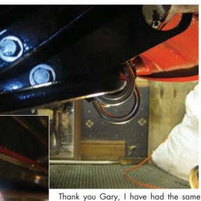
Thank you Gary, I have had the same recovery drivers try and strap the TR7 down on the recovery vehicle bending the track rod ends.
